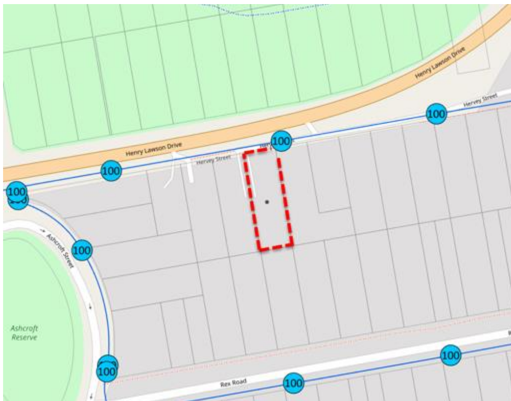
Figure 9 Indicates the location of the nearest mains pressure fire hydrant, with a 100mm mains, outside the neighbouring Lot No.177 Henry Lawson Drive (FRNSW 2026)
